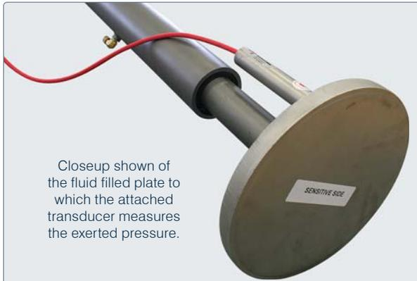
Closeup shown of the fluid filled plate to which the attached transducer measures the exerted pressure.
