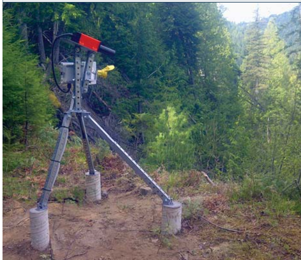
A portable Laser Distance Meter installed in the field with attached survey reflector to enable survey tie-in of the instrument.
