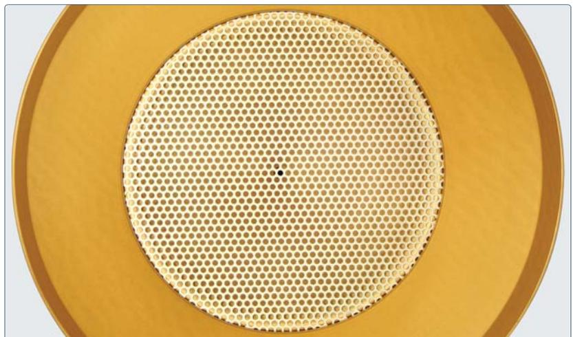
Aerial view of Tipping Bucket Rain Gauge showing filter screen and funnel.
