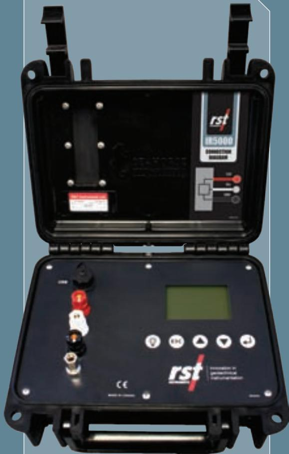
The IR5000 Voltage Transducer Readout reads, displays and logs DC voltage transducers.
